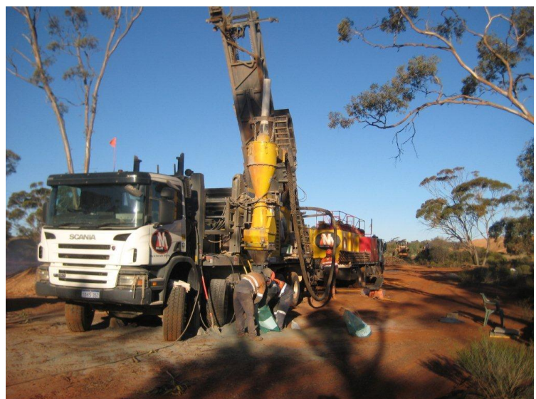
One of the RC drilling rigs currently operating at Bullabulling
