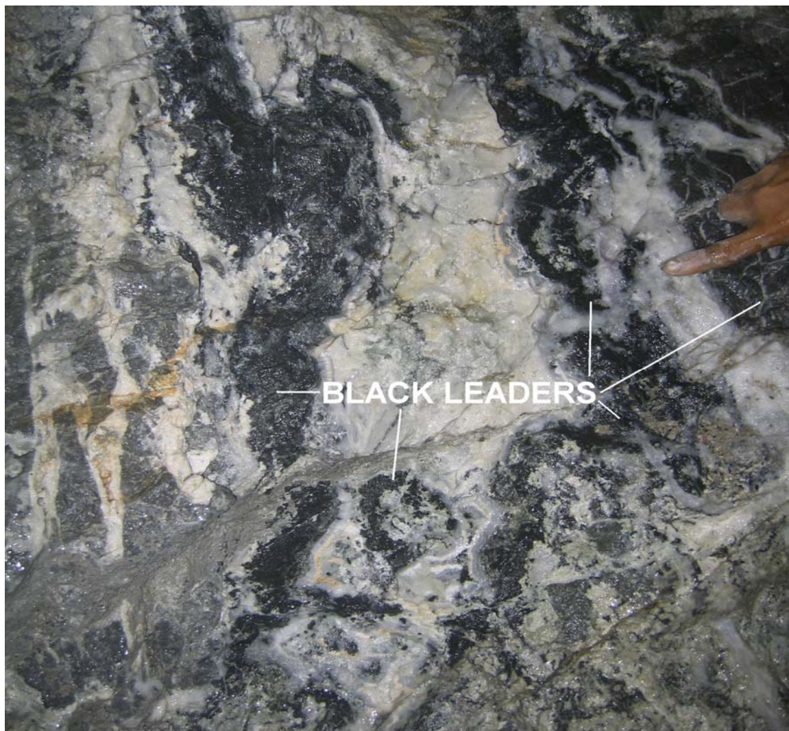
Plate 2. Photograph of “black leader” bands in Central Vein banded and colloform quartz and chalcedony.
