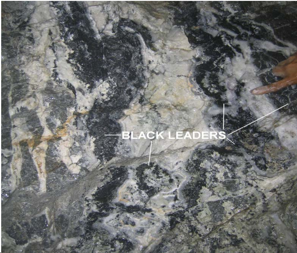
Plate1. Photograph of "black leader" bands in Central Vein banded and colloform quartz and chalcedony.
