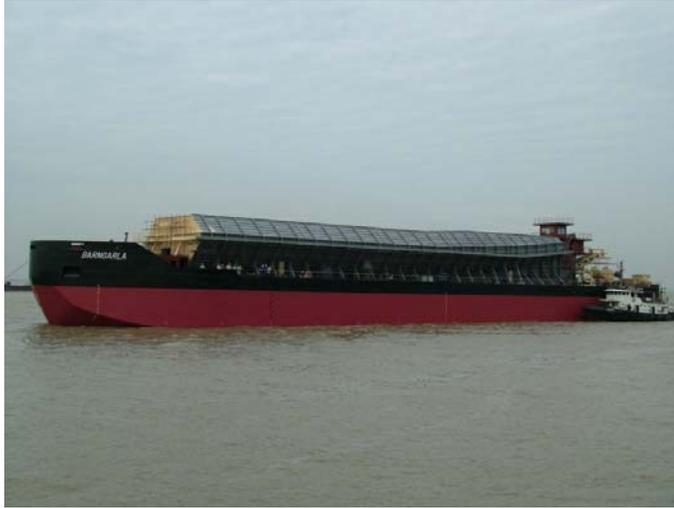
Barngarla, one of the two barges that will be used to trans-ship ore product from the newly-constructed export facilities at the Whyalla port. The barges will carry hematite lump and fines approximately 10 kilometres to a floating offshore transfer terminal which will facilitate loading of Cape-sized ships sitting in the Spencer Gulf. Trans-shipment allows ore transport in large Cape-size ships to maximise the number of potential customers and lower freight costs.
