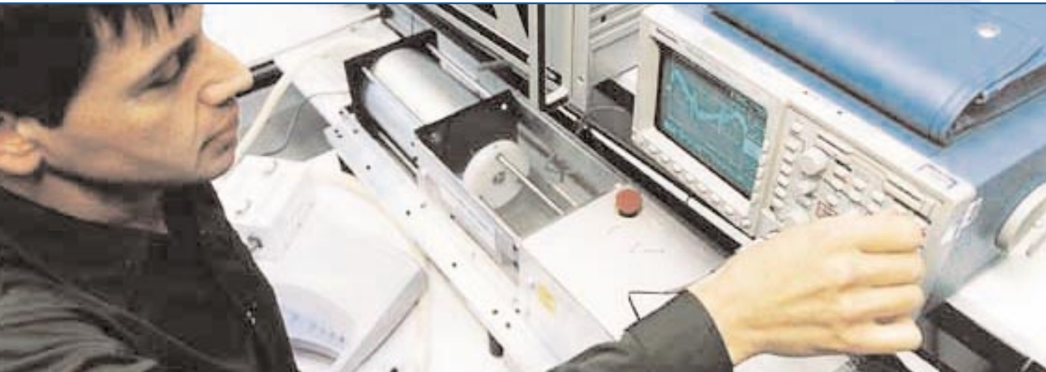
ResMed's custom-built breathing machine accurately simulates breathing patterns to test mask and flow generator function
