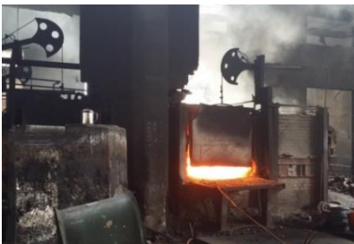
Coal-fired Kiln for Aluminum Melting
