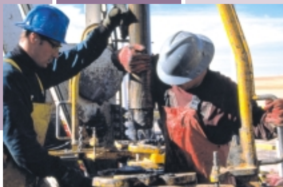
Two oil rig workers, known as "rough necks", prepare a new drill stem at an exploration drilling site.
