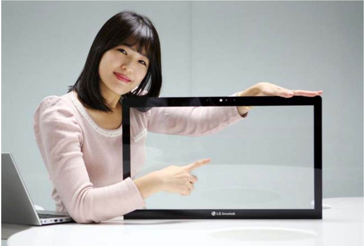
Image 1) LG Innotek staff members present a metal mesh TSP optimized for the medium and large screens in laptops and monitors. Despite the size of the 23 in. screen, the company was able to secure fast response speeds and a competitive price.
