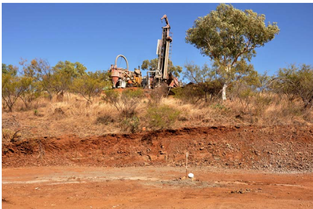
Wahn RC drilling. Rig drilling hole WHRC024 as a scissor hole on WHRC006 in foreground
