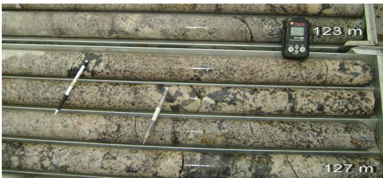
Photograph shows highly mineralised alaskite with smoky quartz
