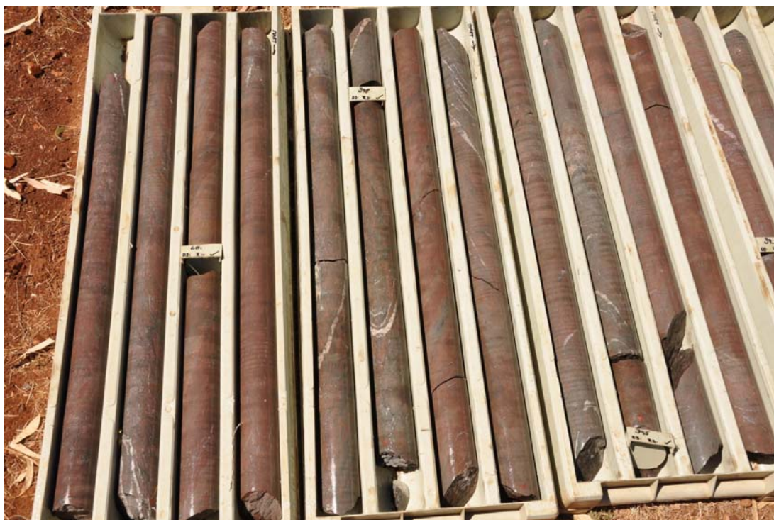
Queens Gift: Drill core from QGD009 showing intense hematite alteration
