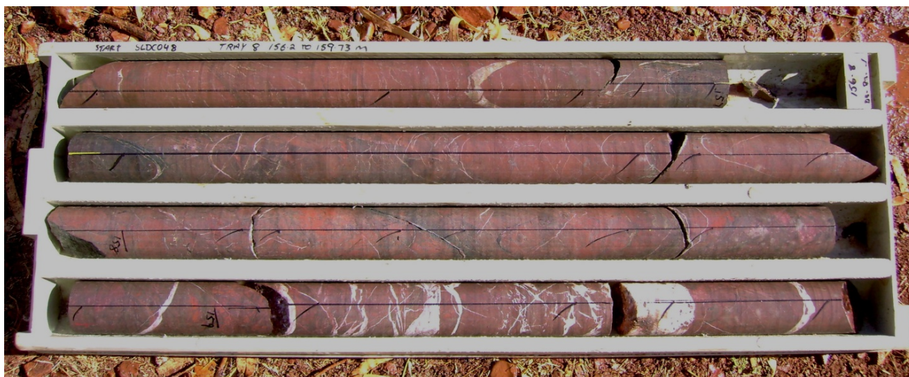
Slance NW Prospect –High grade uranium mineralisation in SLDC048 showing typical hematite alteration of sheared host rock (basalt) and later carbonate-quartz brecciation
