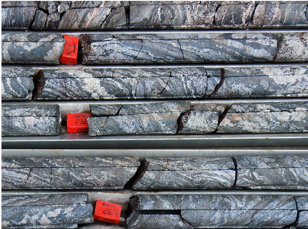
Figure 5: M63 – Medium to coarse-grained dark grey magnetite bands at 23 metres depth (Hole SHID4)
