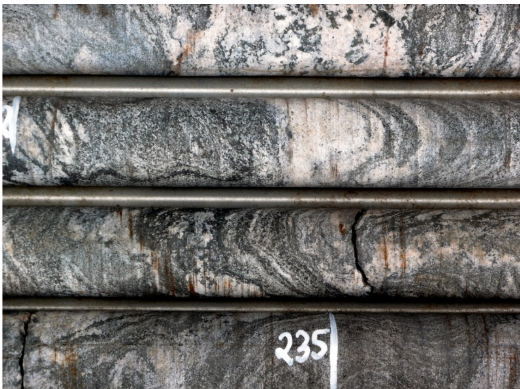
Figure 6: M63 – Fine-medium grained dark grey magnetite bands in folded gneiss 235 metres depth (Hole SHID4)
