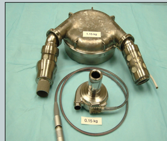
The HVAD is approximately one tenth the size of the HeartMate device
