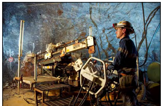
Diamond drilling, underground, at Challenger gold mine, S.A.
