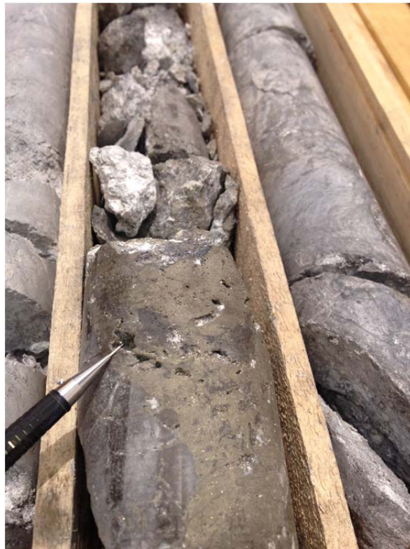
Photo 1: Massive sulphide comprising pyrite and copper minerals, chalcopyrite and chalcocite, in ECHR-25 from 270m down hole.
