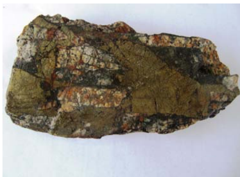
Chalcopyrite/Bornite mineralisation – Kumbruku Prospect
