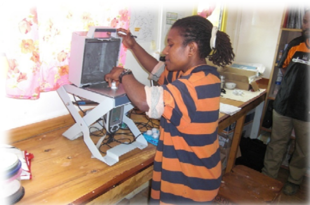
Niton XRF Analyser in Operation at Yandera
