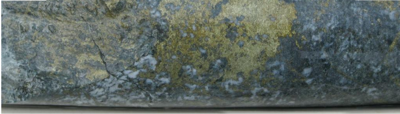
Copper sulphide (predominantly chalcopyrite) in diamond drill core – Yandera Project
