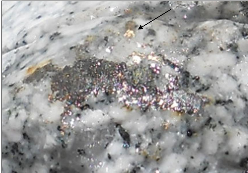
Photo of core from YD536 showing grain of Au in upper centre of the image. Width of the image is ca 2.5 cm. Host rock is a silicified granodiorite porphyry.
