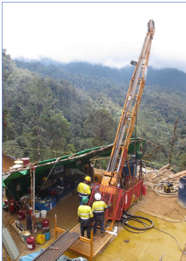
Figure 2: Rig drilling YD 551 on azimuth of 150° (AMG), depressed at -60°
