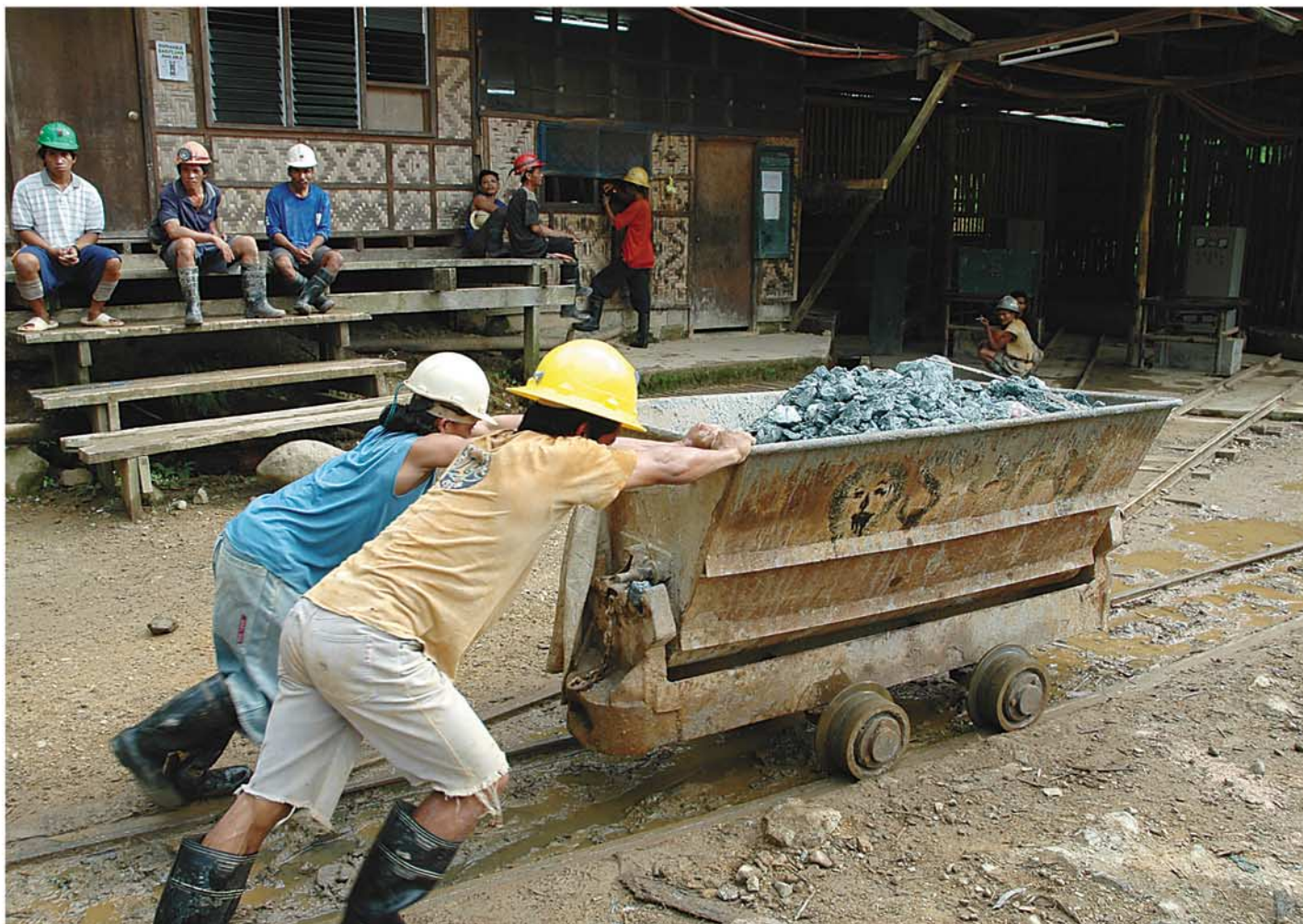
Ore is hand-trammed from the mine to bins, where it is loaded
