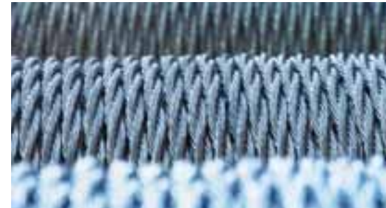
Detail of mining rope.
