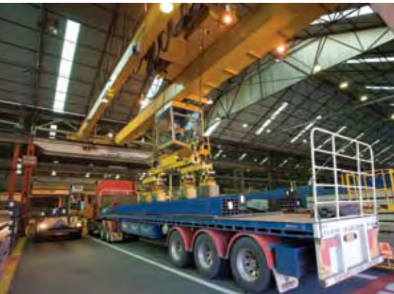
Loading Rectangular Hollow Sections (RHS) at OneSteel's Australian Tube Mill site in Newcastle (NSW).
