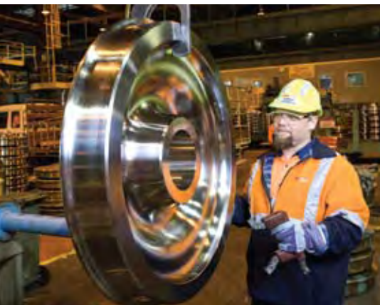
Darren Cummings of Rail Products in Newcastle (NSW) is pictured on the finishing line performing a mag particle test to determine if any cracks are present in the wheel before distribution to customers.
