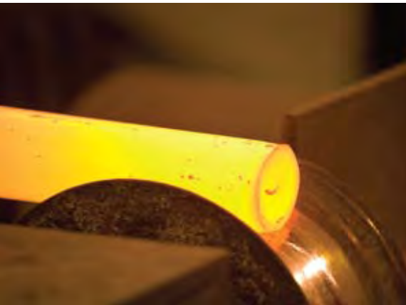
Bar product from OneSteel's Waratah Steel Mill Newcastle (NSW). The bar is transformed into grinding media balls.
