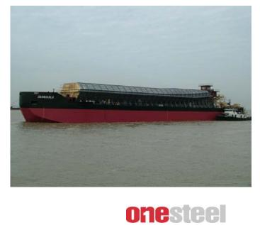
Barngarla, one of the two barges that will be used to trans-ship ore product from the newly-constructed export facilities at the Whyalla port. The barges will carry hematite lump and fines approximately 10 kilometres to a floating offshore transfer terminal which will facilitate loading of Cape-sized ships sitting in the Spencer Gulf. Transshipping allows ore transport in large Cape-size ships to maximise the number of potential customers and lower freight costs.
