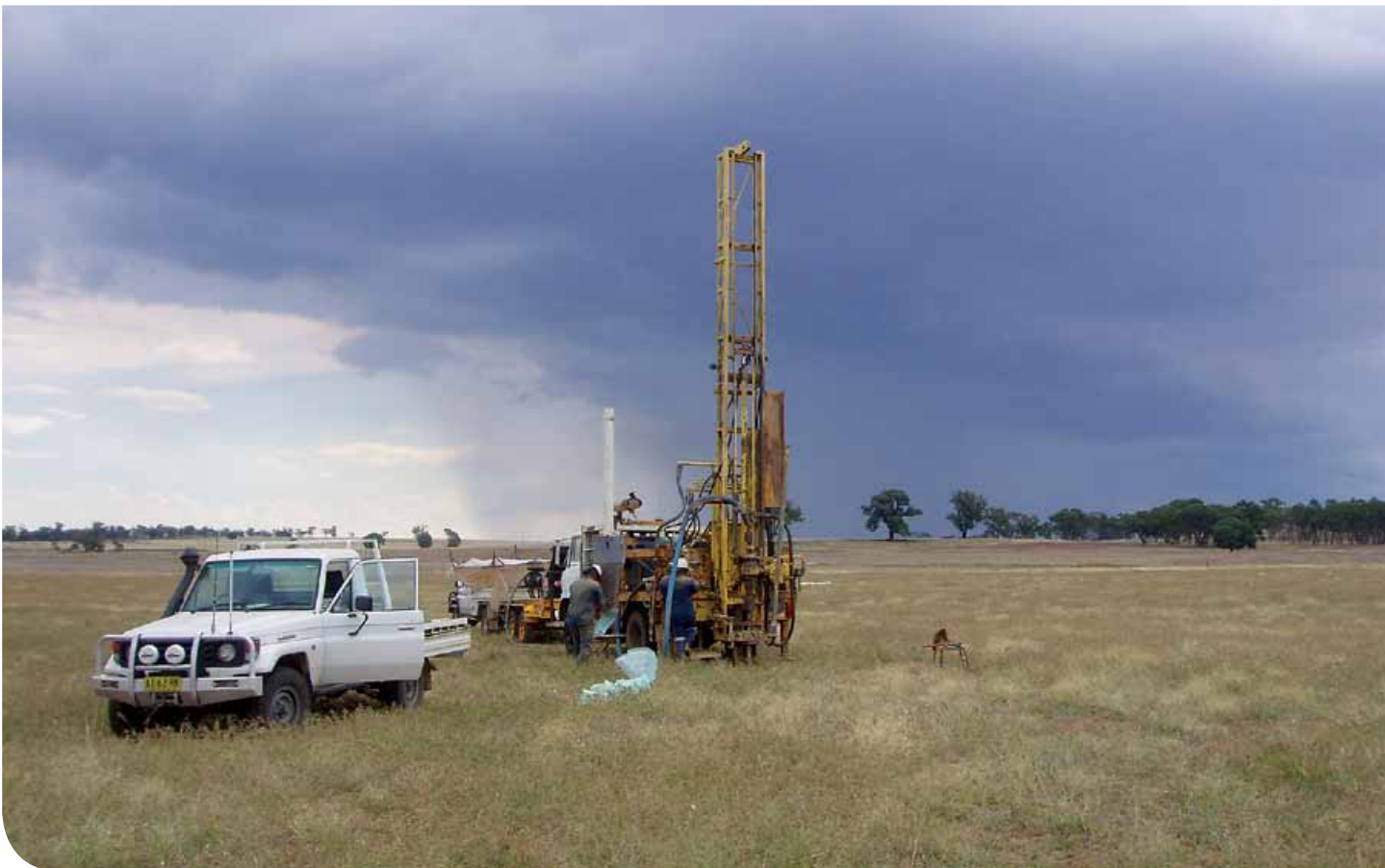
Aircore drilling - Mt Leadley
