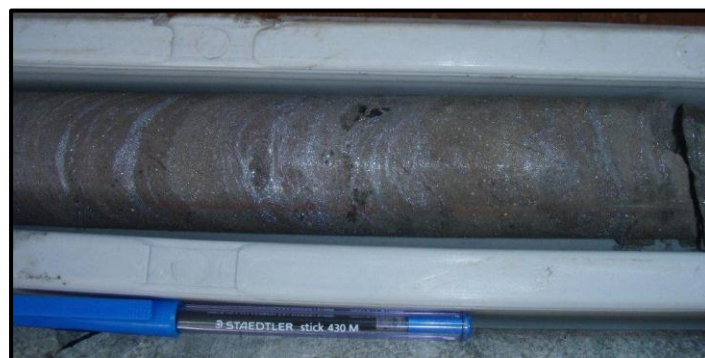
Detail of massive lead-zinc sulphides in hole HRD042W1 – approx. 327m down hole depth
