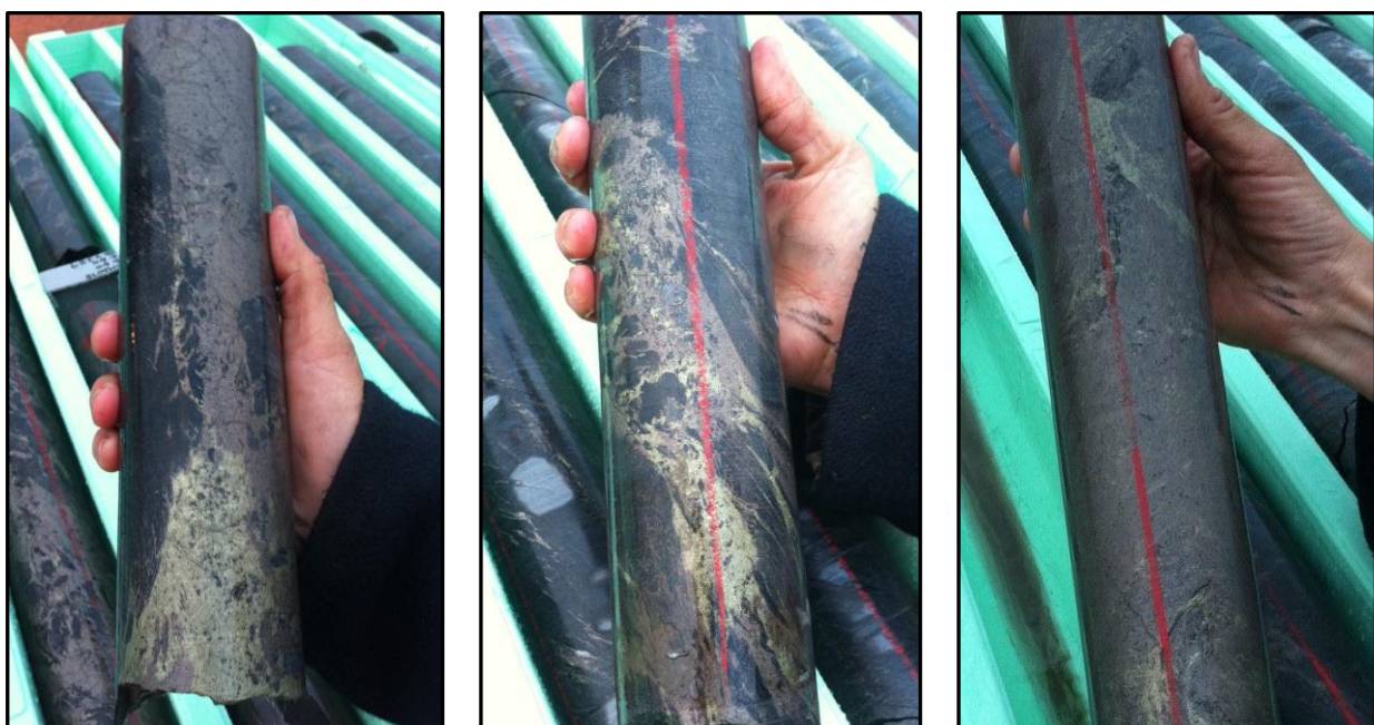
Selected core photos from matrix and massive iron and copper sulphide zone in hole NMD075
