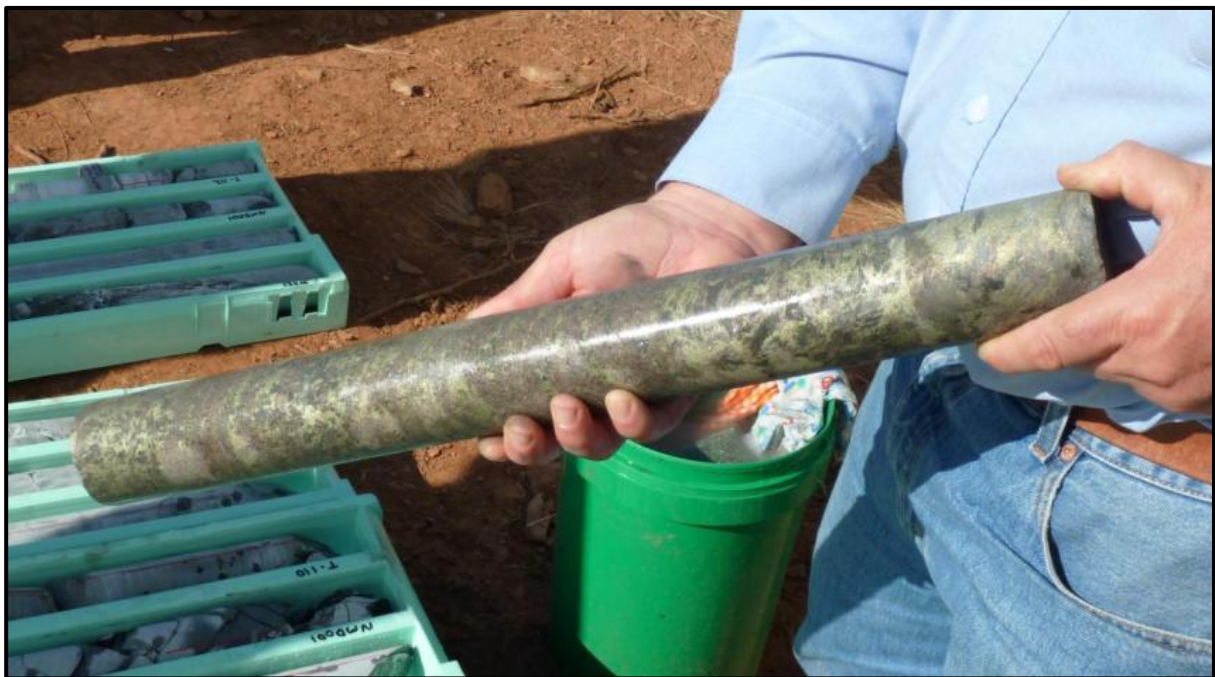
Massive sulphide mineralisation – Nymagee Copper Deposit
