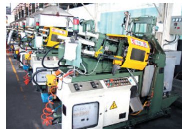
Die-casting zipper sliders
