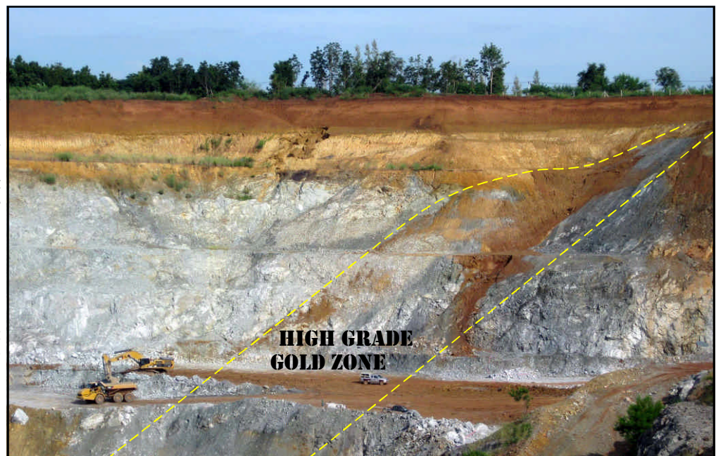
C North Pit showing exposed high grade gold zone
