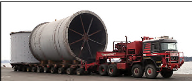
SAG Mill and Ball Mill shells arrive by sea and are road transported to Chatree where the new Ball Mill heads are waiting
