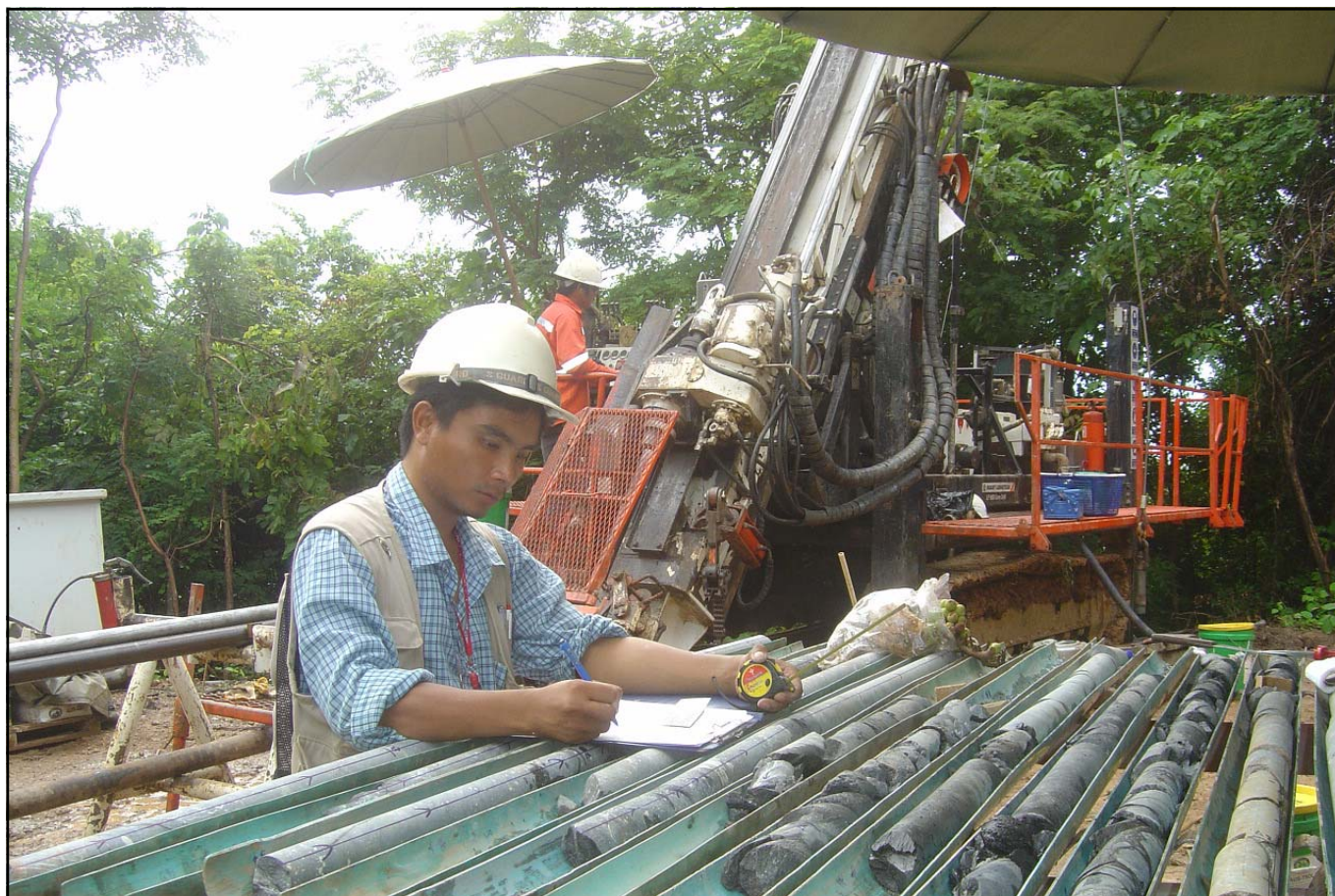
Logging drill core is an essential task on every project
