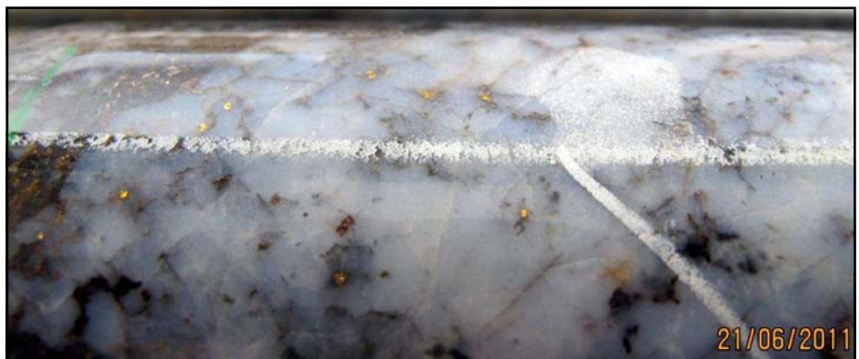
Visible gold in drillcore (NQ core size, 47.6mm diameter) from Challenger gold mine, South Australia
