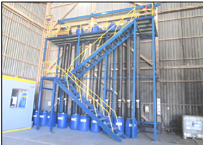
Column leach testwork on-site at Nueva Esperanza
