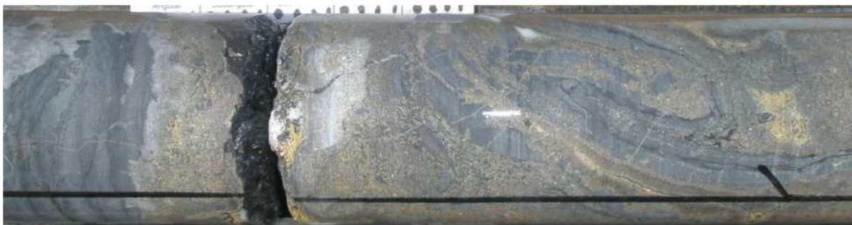
Figure 7 Drill core of zinc mineralisation from JB001
