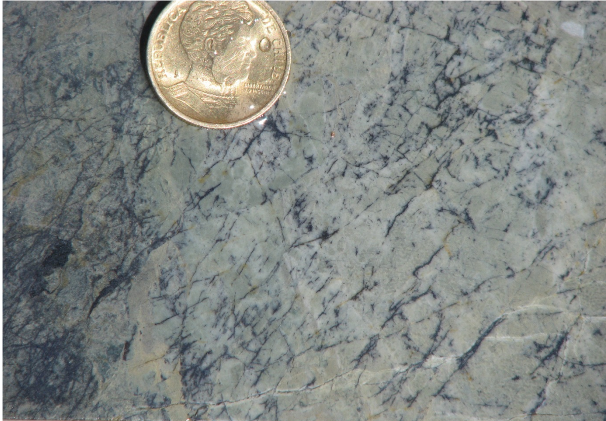
Figure 6 Drill core San José - MSJ-04, 364.5m, 5%Cu, 48.3g/t Ag
