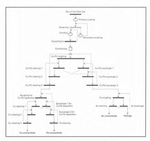
Figure 8.1 Ore Processing Flowsheet for the Damajianshan Mine
