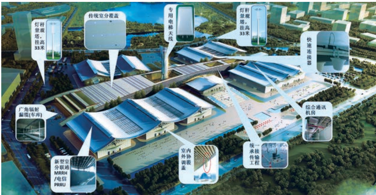
▲ Diagram of DAS coverage program for Shijiazhuang International Convention Center
