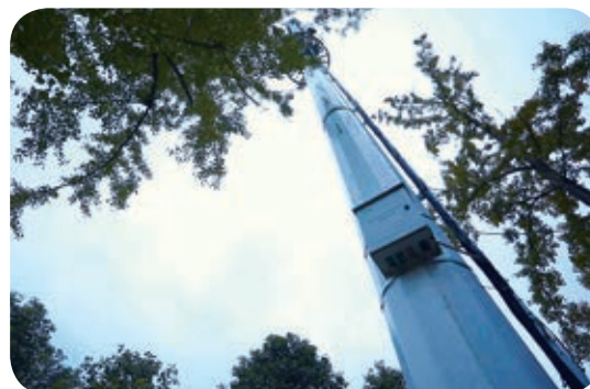
▲ Air quality monitoring equipment installed on tower poles
