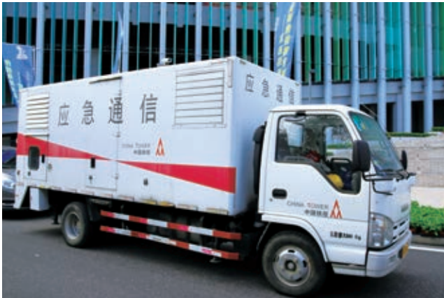
▲ Emergency support power supply vehicles
