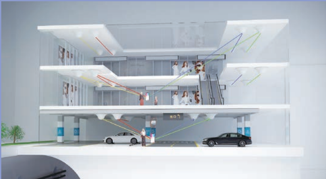
Diagram of 5G passive distributed MIMO technology in high-capacity building scenarios
