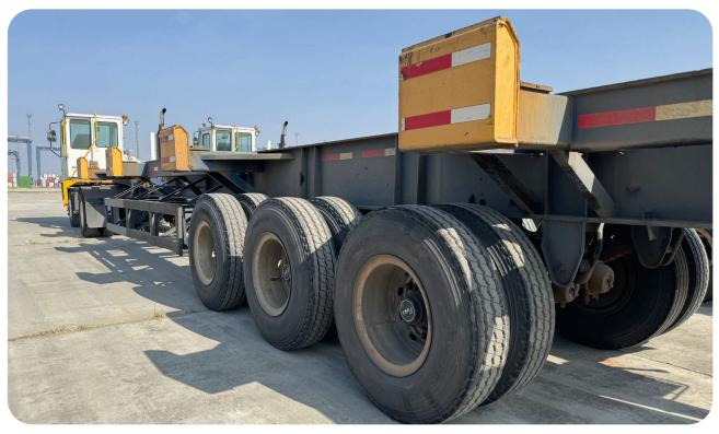
Re-treaded tyres installed at the terminal trailer, Hutchison Ports MITT
