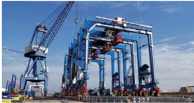
Xiamen Ocean Gate Terminal introduced a new generation of electric gantry cranes.
