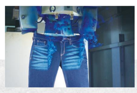
Laser technology — saving five to seven litres of water per garment piece on average - was used in the production of 12.6 million pieces of denim wear in our factories during the year.
