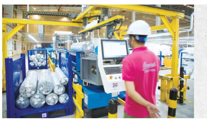
At our denim factories, incoming fabric rolls from suppliers are machine sorted into racks before they are distributed to the corresponding workstations
