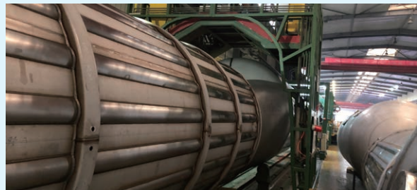
Automatic Welding System for Reinforcing Ring of Special Tank Box
