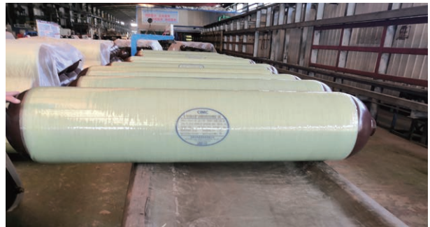
CNG vehicle-mounted tank
