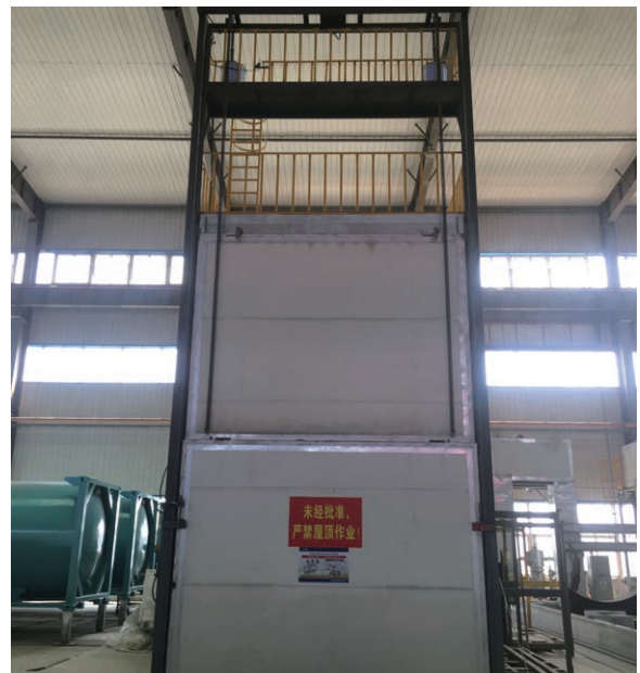
Double-layer vacuumizing drying room
