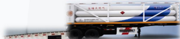
高压氢气集装管束及运输车 High-pressure Hydrogen Tube Container and Trailer
