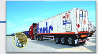
High-pressure Hydrogen Tube Container and Trailer
