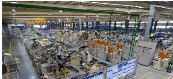
Automated Robotic Welding
