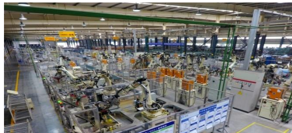
Automated Robotic Welding
