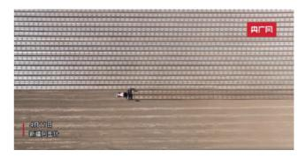
The Dongfanghong autonomous tractor, utilizing precise Beidou satellite navigation positioning, conducts precision sowing along pre-set routes. It achieves complete mechanization in laying drip irrigation tapes and plastic mulch, with a straight-line error of less than 2 cm. Compared to traditional sowing methods, this approach saves over 50% of cotton seeds. enhances land utilization, and facilitates later mechanized field operations and harvesting.
