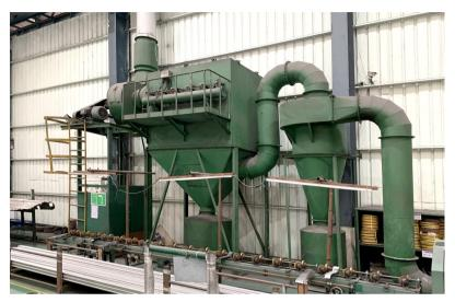
Production plants equipped with dust collectors with filter bags
