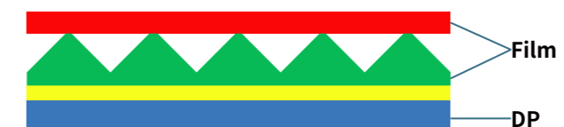
Schematic diagram of optical film and diffuser plate bonding (Film: optical film; DP: diffuser plate)
