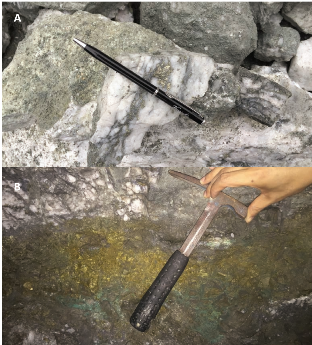
Figure 4-1: Auriferous quartz veins are commonly associated with A: pyrite and B: chalcopyrite/malachite
