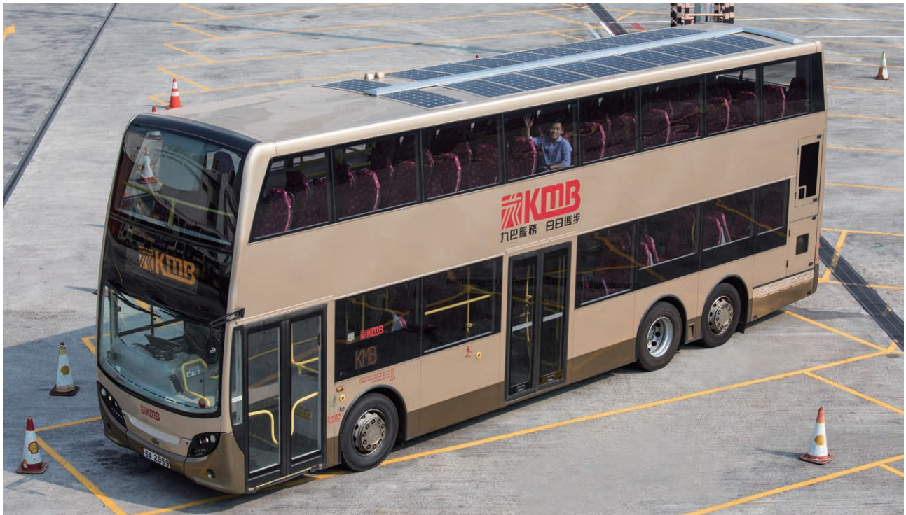
KMB introduced the first in-house developed bus equipped with a solar power system 九巴自行研發首部配備太陽能發電裝置的巴士
